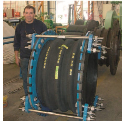
Figure 25 – Triple Arc Expansion Joint
