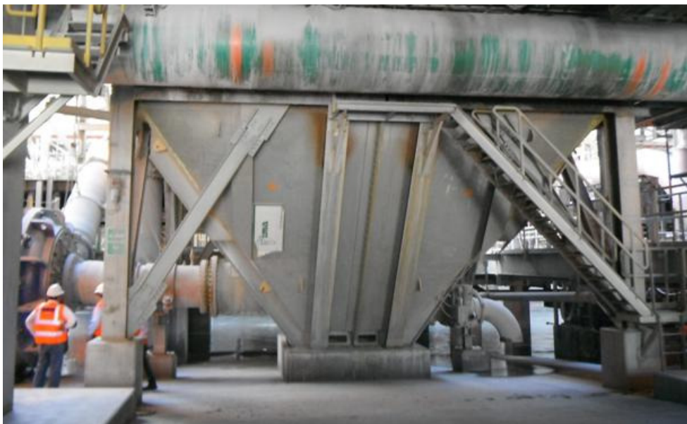
Figure 35 – Suction Sump Hopper, MCR® 650 Mill Circuit Pump
