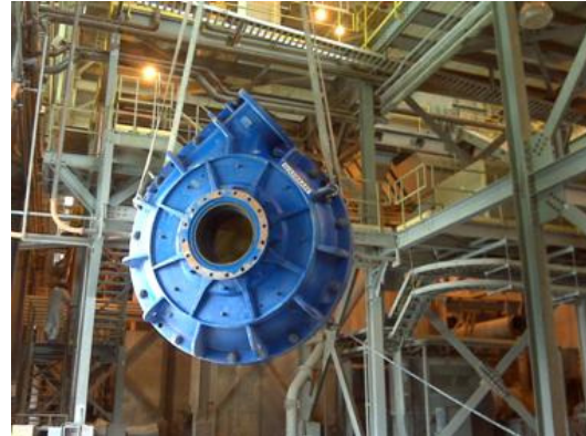
Figure 55 – Warman® Pump, Wet End Assembly
