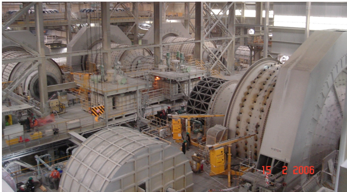
Figure 1 – Grinding plant, Sag Mill and Ball Mills Circuit
