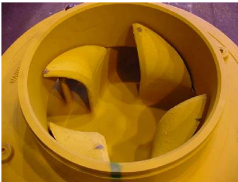
Warman patented flow inducer impeller vanes ( scoops ) Figure 5
