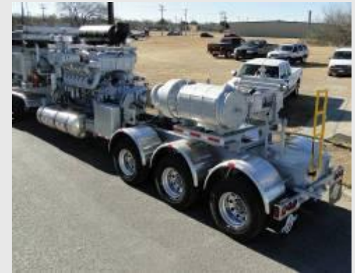
Destiny™ TWS 2500 frack pump installed on customer pump unit
